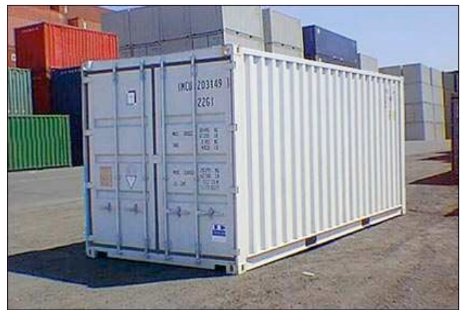
Figure 1: 20-foot ISO 668 Shipping Container
